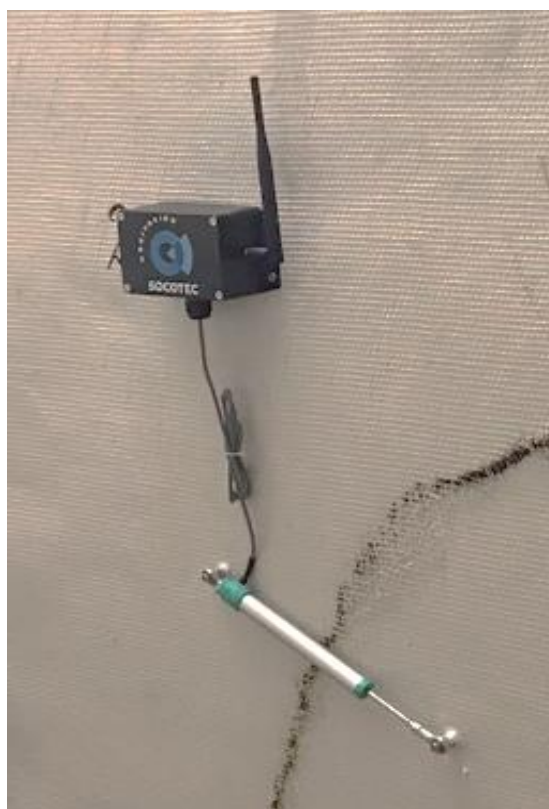
Figure 12 : Photo of a NodeLog installation with 100mm GEFran transducer
